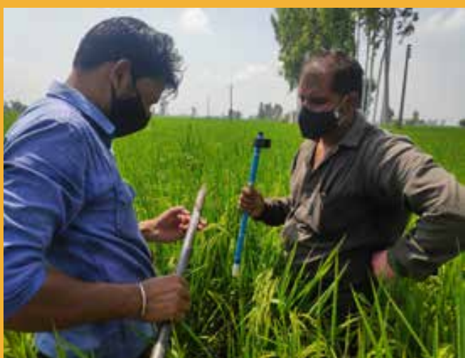
J-PAL South Asia surveyors installing tensiometer to measure soil moisture in Patiala, Punjab.
